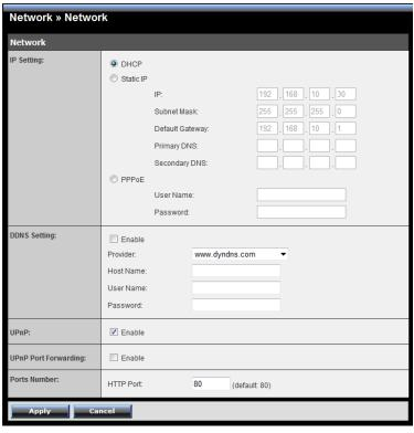
• **IP Setting:** This item allows you to select the IP address mode and set up the related configuration.
